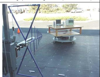
Photograph I-3 - Horizontal Polarization (30MHz - 1 GHz)
