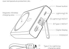
1 and 2 are both two-way fast charging ports. It is recommended to use the special built-in cable of 3OVROOM. The built-in cable lightning head 1 is inserted into the 1 interface position of the power bank, and Type-C head 2 is inserted into the 2 interface position of the power bank.
