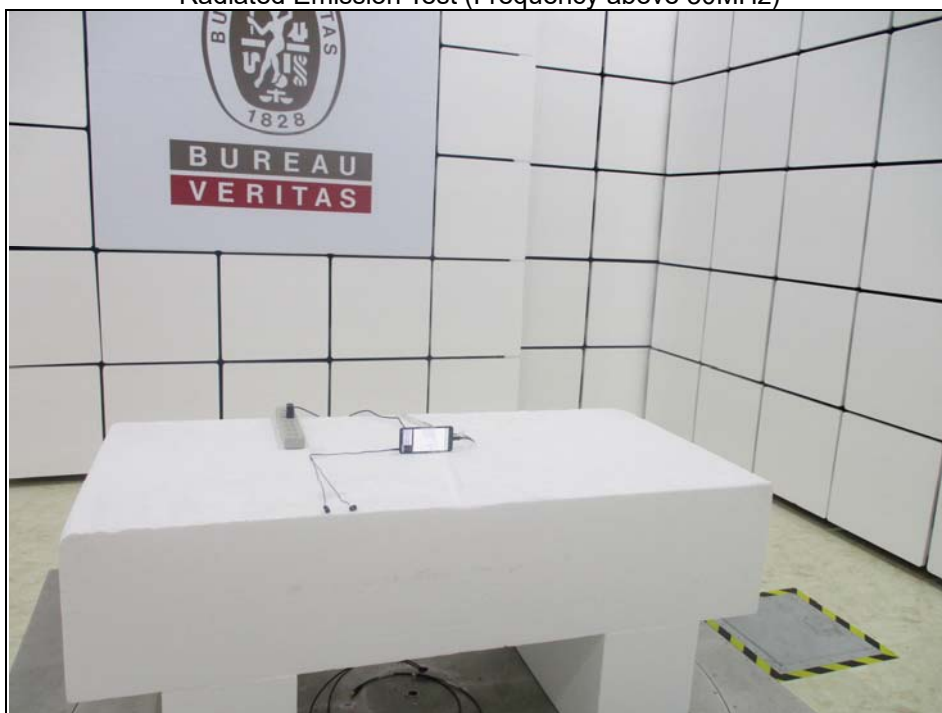
Radiated Emission Test (Frequency above 30MHz)
