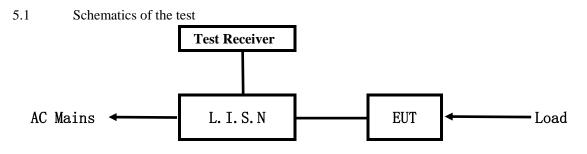
EUT: Equipment Under Test
