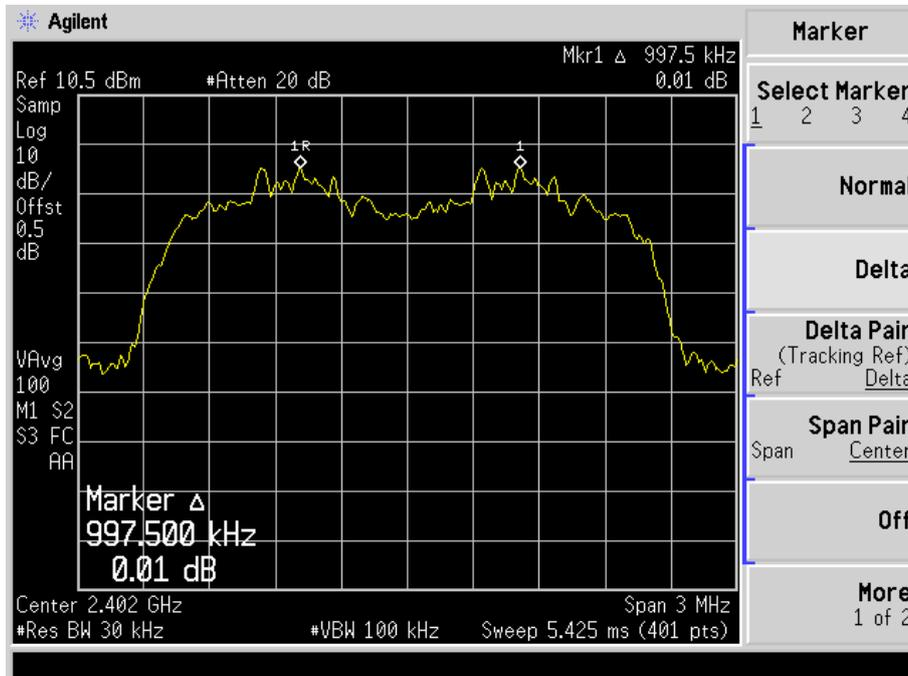
Channel Spacing (Middle CH=1MHz)
