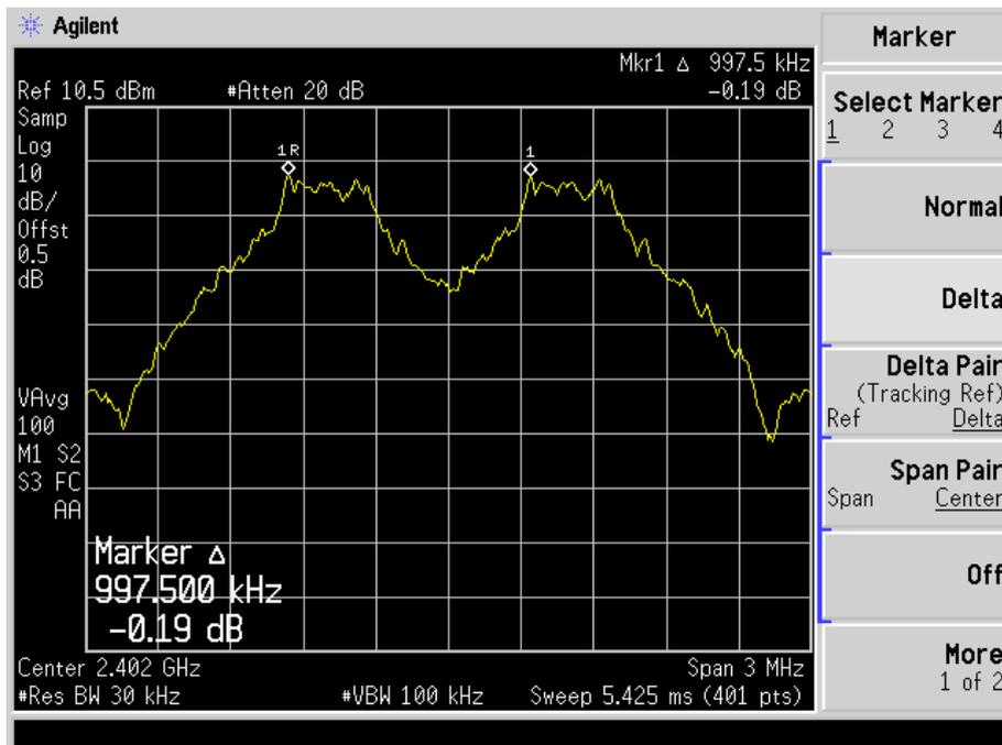
Channel Spacing (Middle CH=1MHz)
