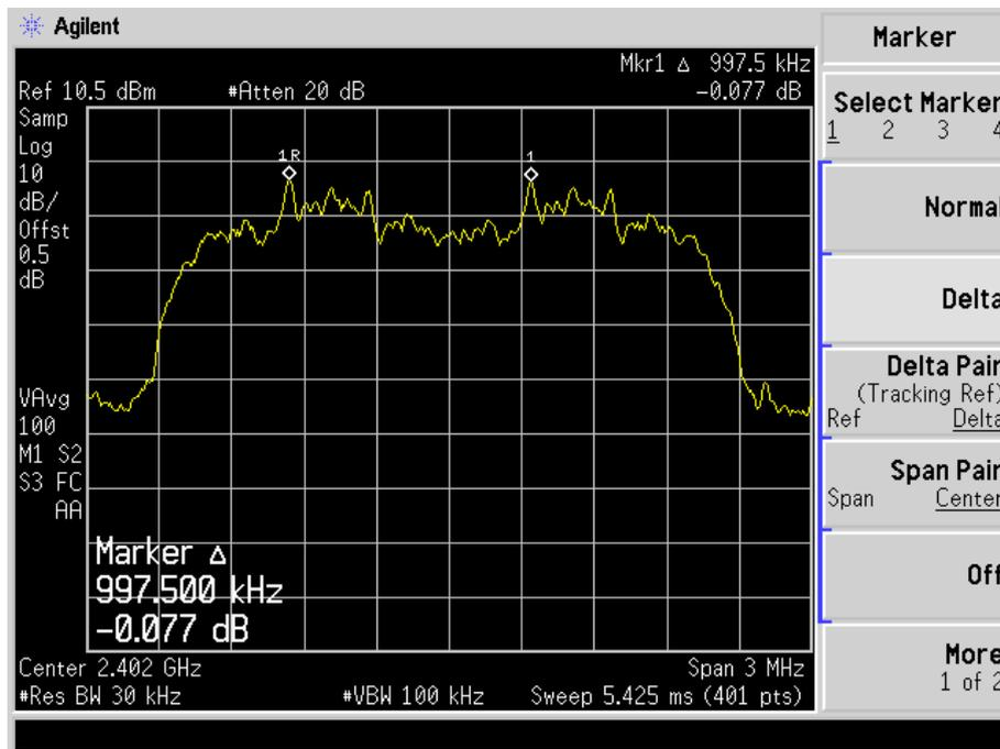
Channel Spacing (Middle CH=1MHz)
