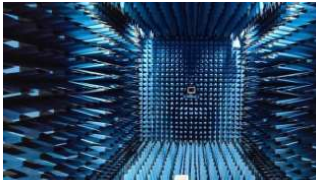
Figure 2: Geometry of Anechoic Chamber for Radiation patterns.
