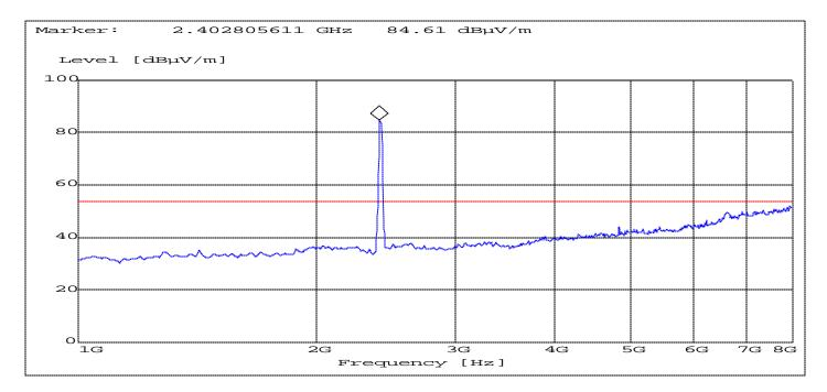
NOTE: The marked peak is the carrier frequency. Frequency resolution is not fine enough to show the exact frequency of the carrier, refer to plots under EIRP.
