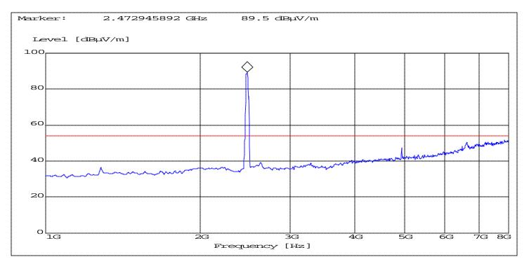
NOTE: The marked peak is the carrier frequency. Frequency resolution is not fine enough to show the exact frequency of the carrier, refer to plots under EIRP.
