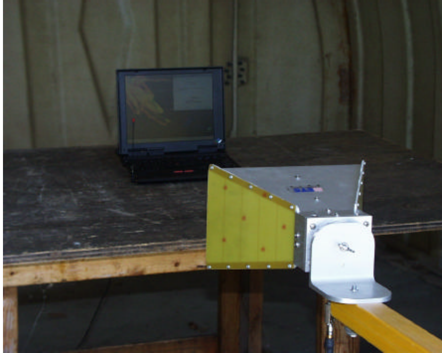
Above 1GHz Radiated Emission Setup
