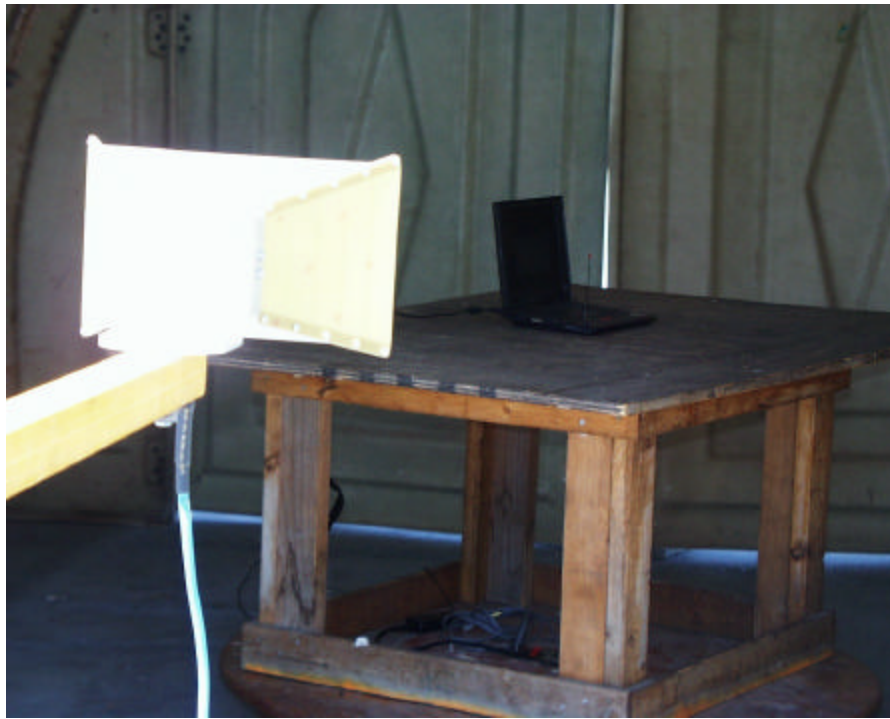
ERP Setup @ 1900 MHz
