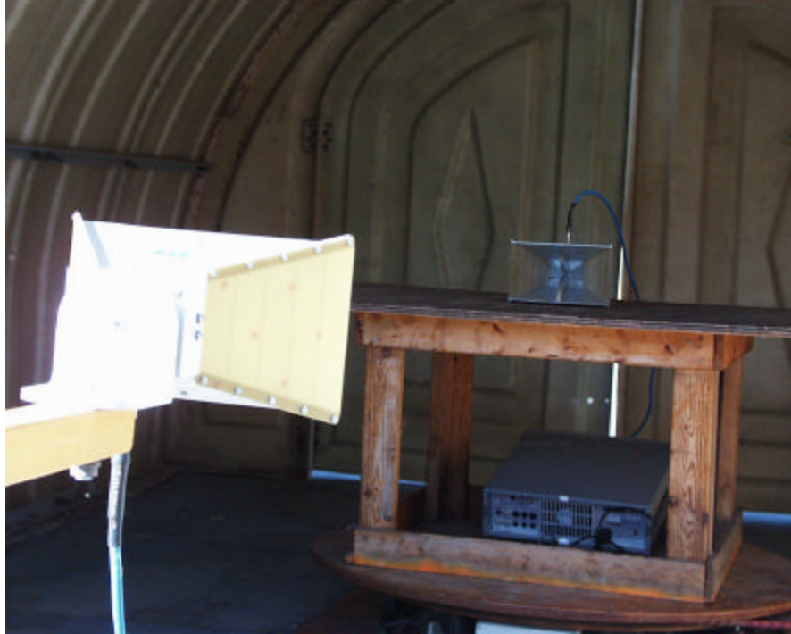
Substitution Method @ 1900 MHz
