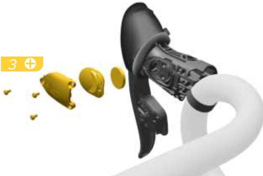
Install a new CR2032 battery with the positive + sign facing outward. Wipe the gasket with a lint-free rag so it is free of dirt and debris, then install the gasket and battery hatch.
