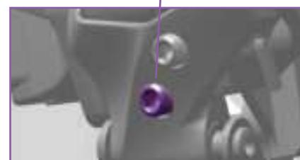
**If the chain drops inboard when shifting to the small chainring:** With the front derailleur in the inboard position, rotate the low limit screw clockwise 1/8 turn. Repeat until the chain no longer drops from the chainring.
