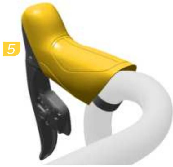
Gently tighten the battery hatch screws until they are hand tight.
