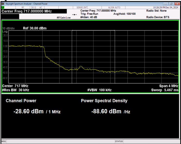
Band12 QPSK BW=1.4MHz Channel=23173 RB Size=6 Position=#0 Extended
