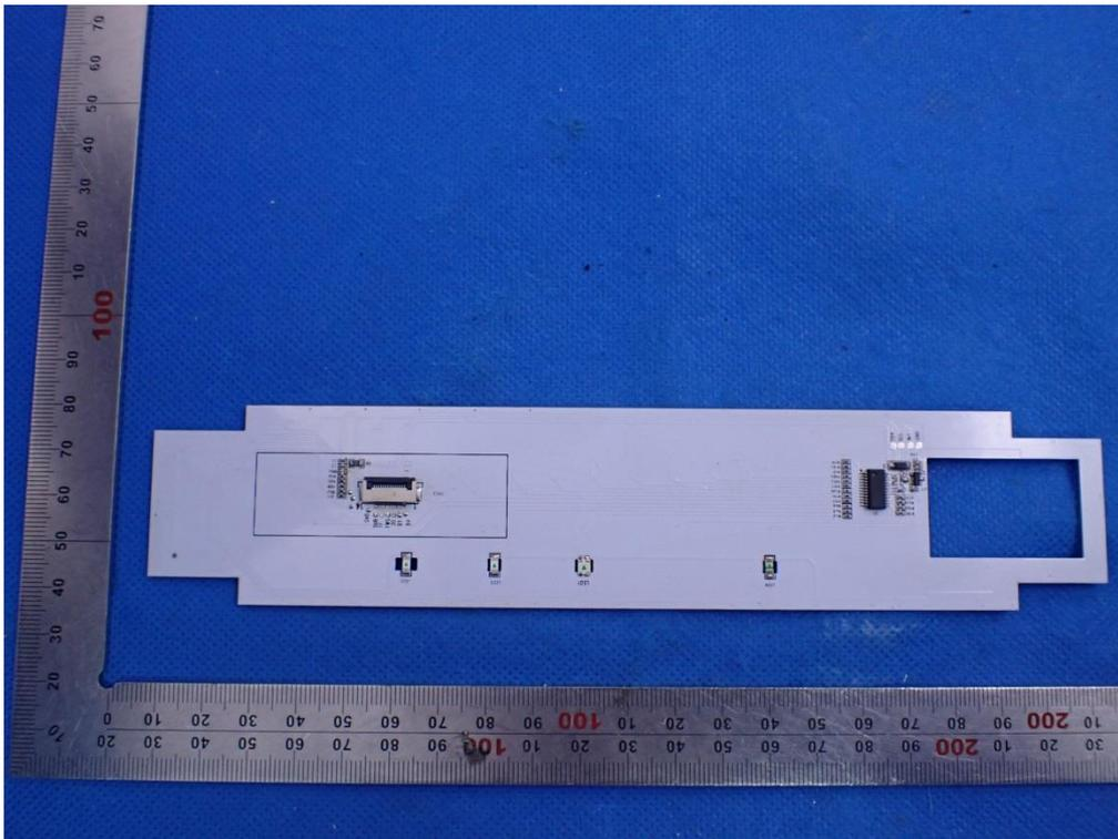
INTERNAL VIEW OF EUT-6(NFC Antenna)
