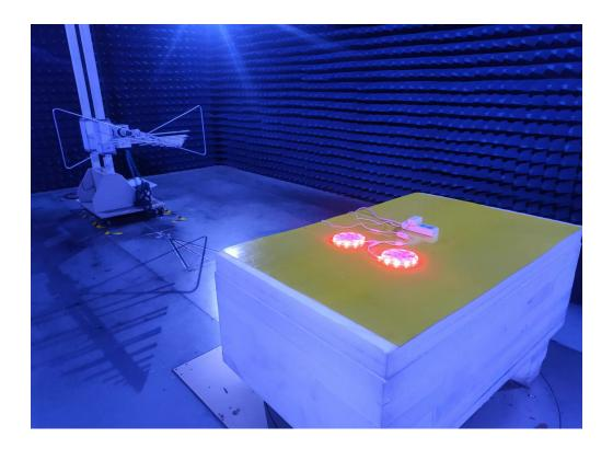
Photo of Radiated Emission Measurement (Above 1G)
