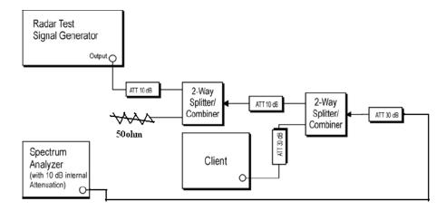
Figure 3-2: Radar Waveform Calibration Conducted Test Setup
