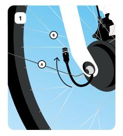
↑ The motor cable must go around the back of the fork, between the fender stay (A) and the spokes (B).
