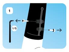
↑ Remove the two screws on the side.
