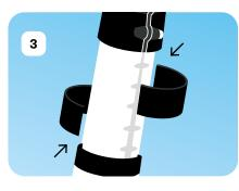
↑ Place one or the two spacers, loosen the screw and slide the handlebar down.
