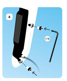
→ Tighten the two screws into the motor cable cover. Make sure both of them are secure.
