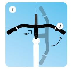
↑ Rotate the handlebar so that it forms a 90° angle with the bike frame.
