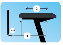
↑ Loosen both screws underneath the saddle, adjust the seat to your preferred position, and tighten the screws.
