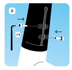
↑ Tighten the screws just enough to hold the handlebar in place. We'll be adjusting the height later on.
