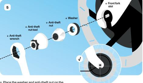
↑ Place the washer and anti-theft nut on the left side of the wheel and tighten using the anti-theft wrench.
