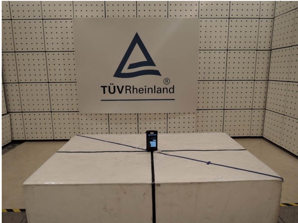
Photograph 1: Set-up for Spurious Emissions (Front View)
