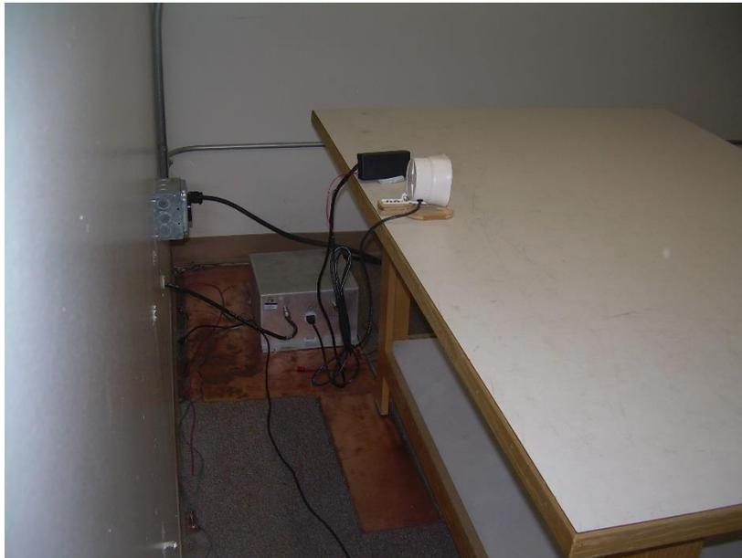
**Photograph 8 - Back View Conducted Emissions Worst Case Configuration**
