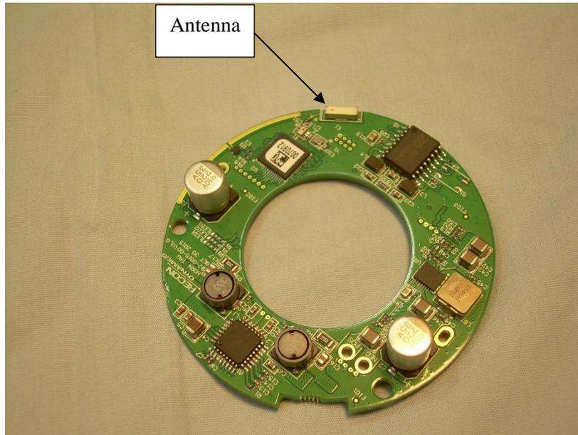
**Photograph 13 – Front Side of the PCB**
