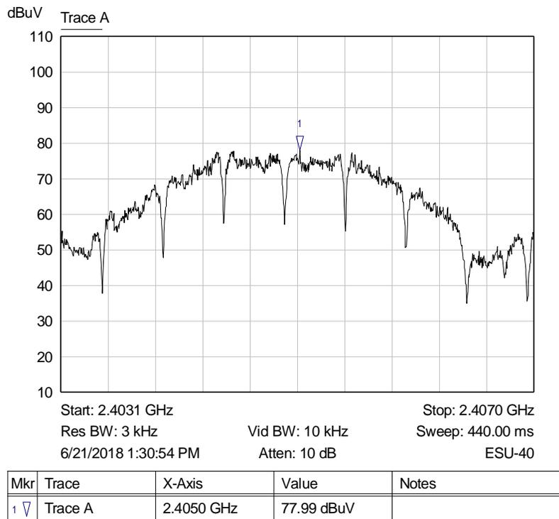
**Graph 9: Lowest Channel 3 kHz PSD Plot**
