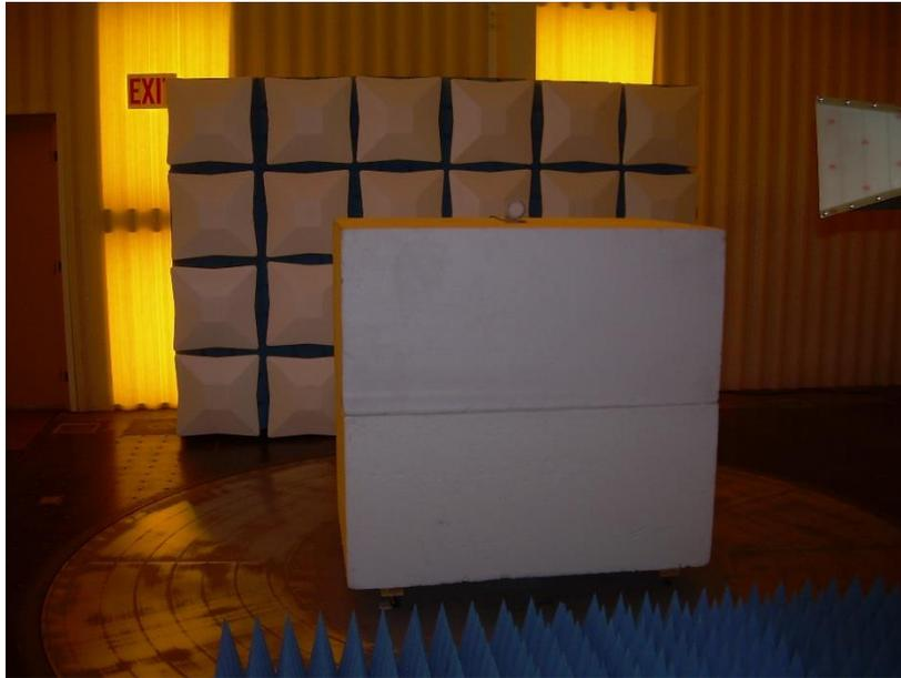
**Photograph 5: Front View Radiated Emissions – Above 1000 MHz**
