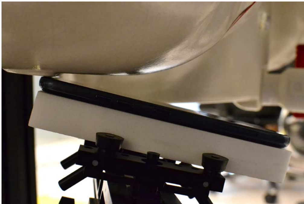
SAR Test Setup Photo 2 – Right Tilt
