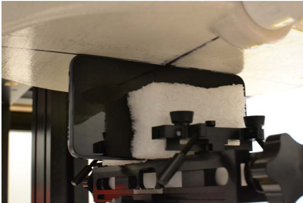
SAR Test Setup Photo 18 – Left Side at 0 mm
