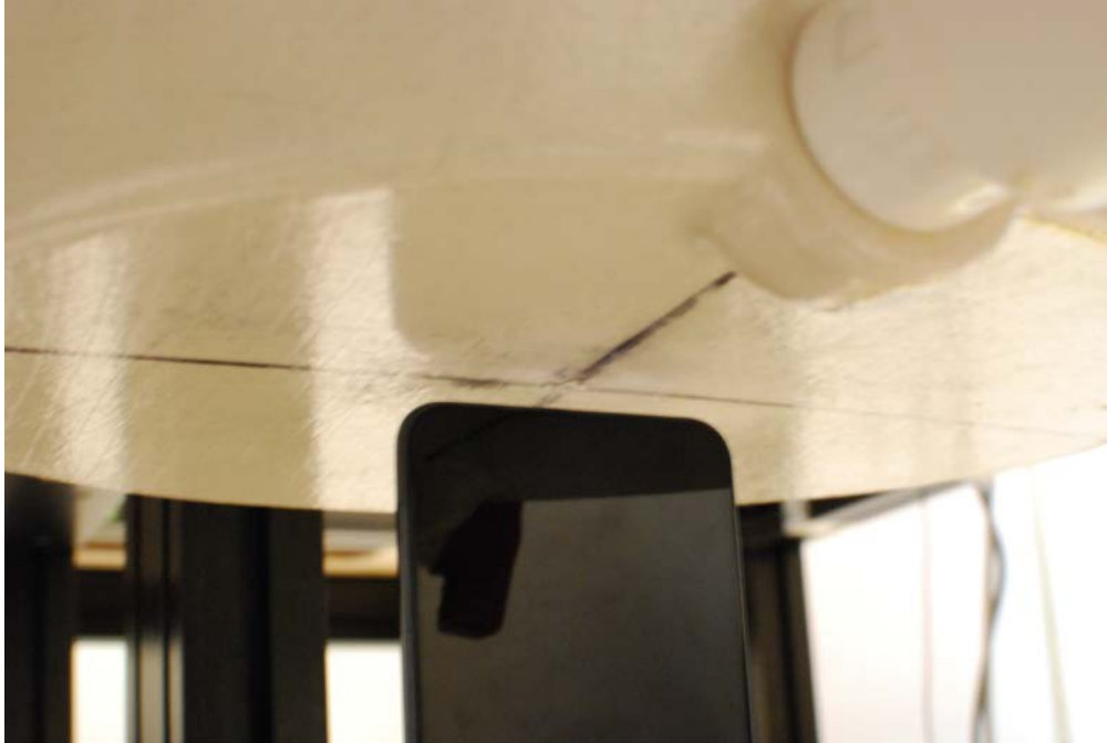
SAR Test Setup Photo 13 – Bottom Side at 4 mm
