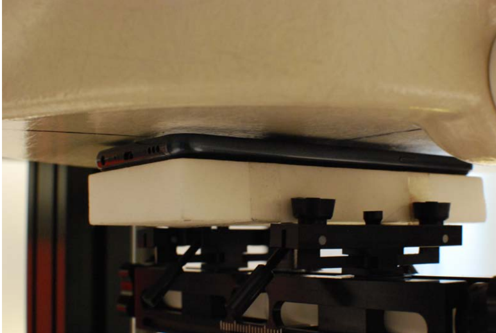
SAR Test Setup Photo 9 – Front Side at 3 mm
