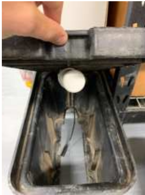
Figure 3: shows LORIKEET with Antenna positioned closest to lid opening point
