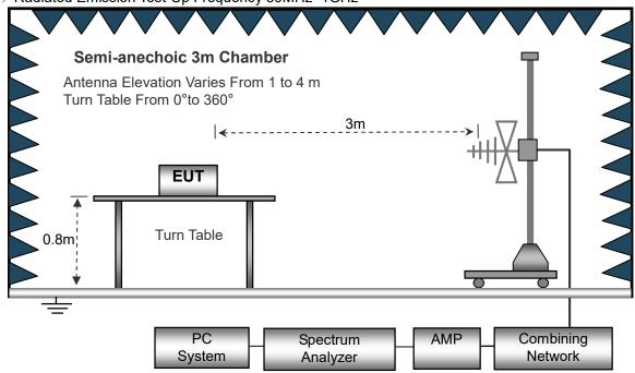
(C) Radiated Emission Test-Up Frequency Above 1GHz
