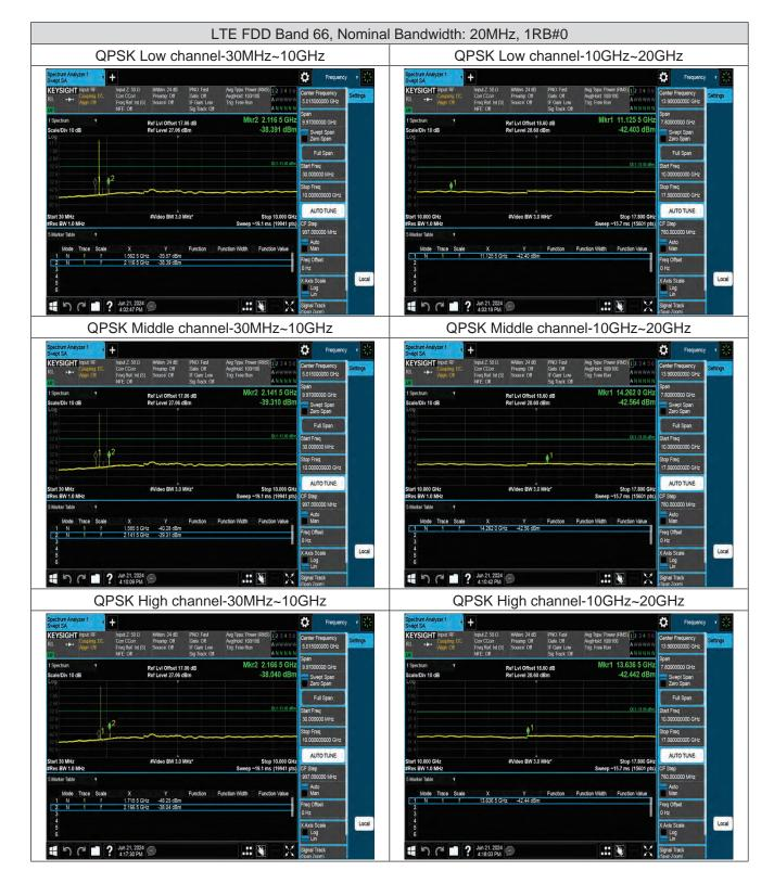
Note: All modes have been tested and we found QPSK modulation, 1 RB#0 test mode has the worst test result. Only record the worst test result.
