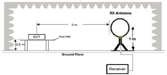
(2) Radiated Emission Test-Up Frequency 30MHz~1GHz
