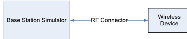
Figure 9-3 Power Measurement Setup
