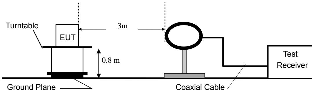
Radiated Emission Test Set-Up, Frequency Below 1GHz
