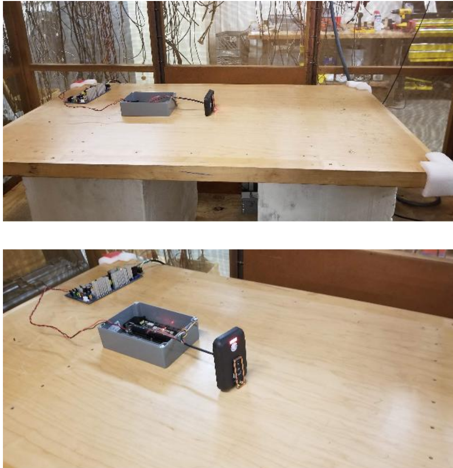
Figure 6: Conducted Emissions Test Setup Photograph(s).
