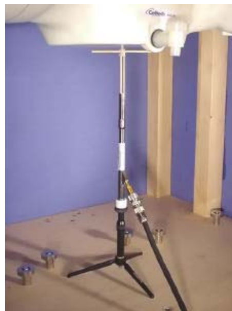
900MHz System Check Setup
