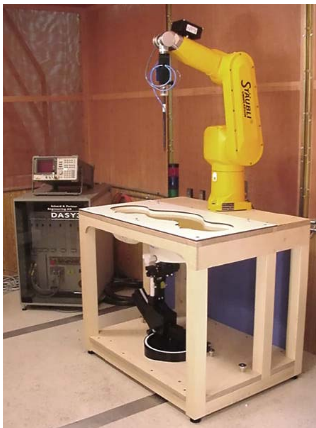
DASY3 SAR Measurement System with SAM phantom
