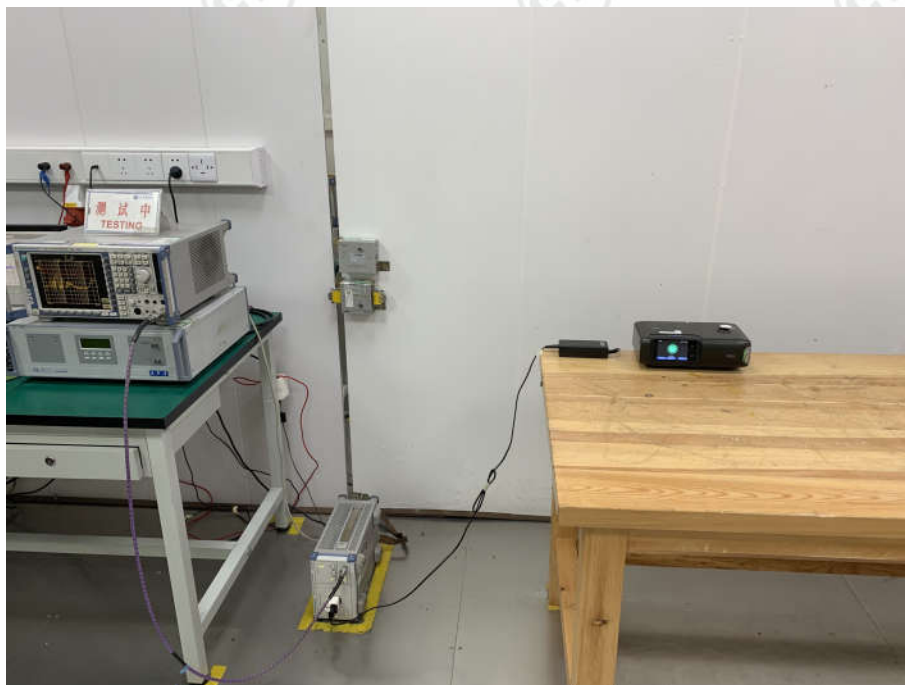
Conducted Emissions Test Setup
