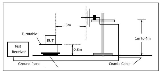
(c) For radiated emissions above 1000MHz
