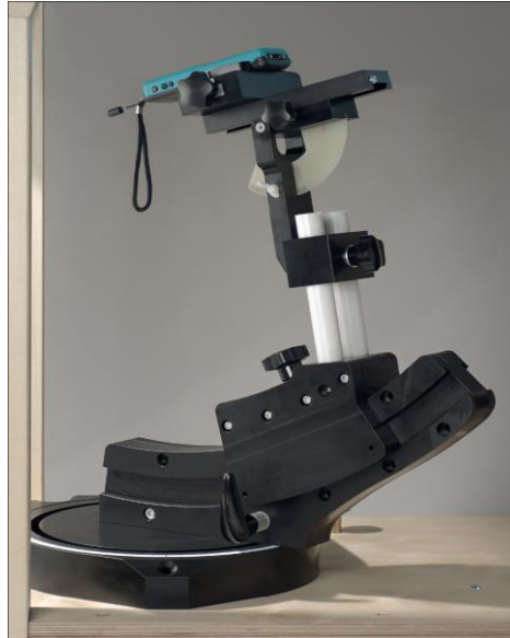
F-2. Device Holder for Transmitters
