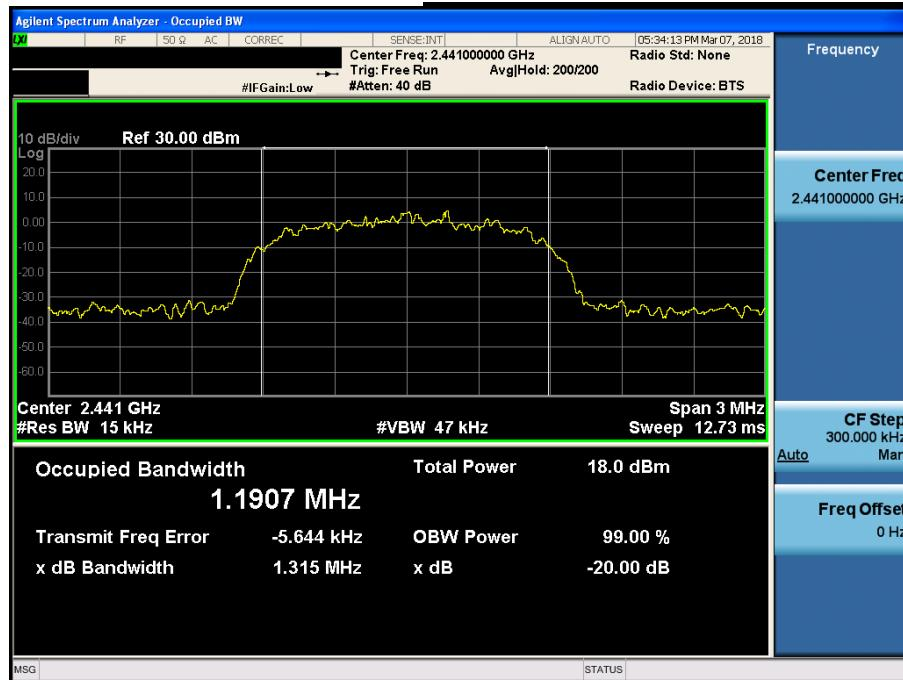
**20 dB Bandwidth****Highest Channel & Modulation : 8DPSK**
