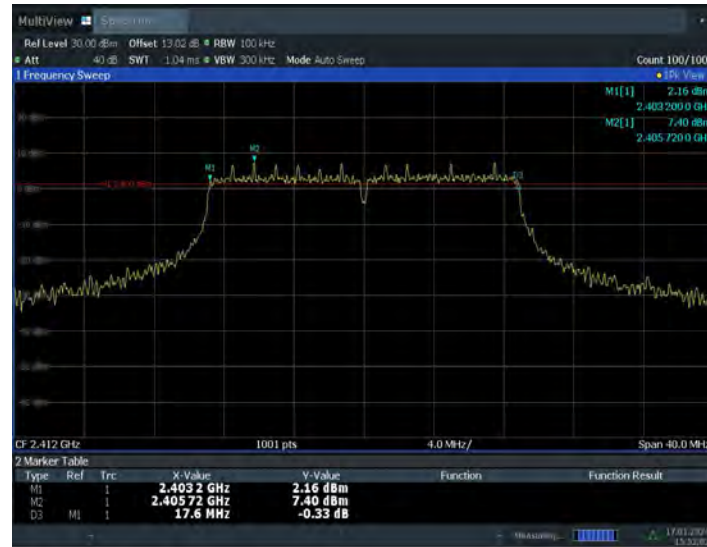
Fig.A.4.7 DTS Bandwidth (802.11n-20MHz, Ch 1)
