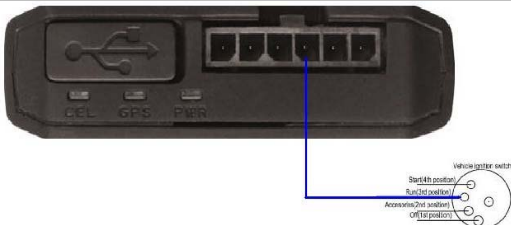
Figure 6. Typical Ignition Detection
