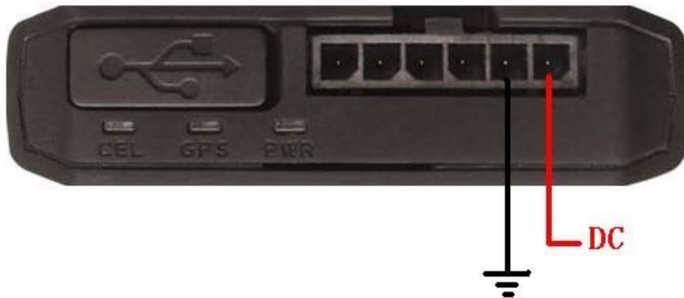
Figure 5. Typical Power Connection
