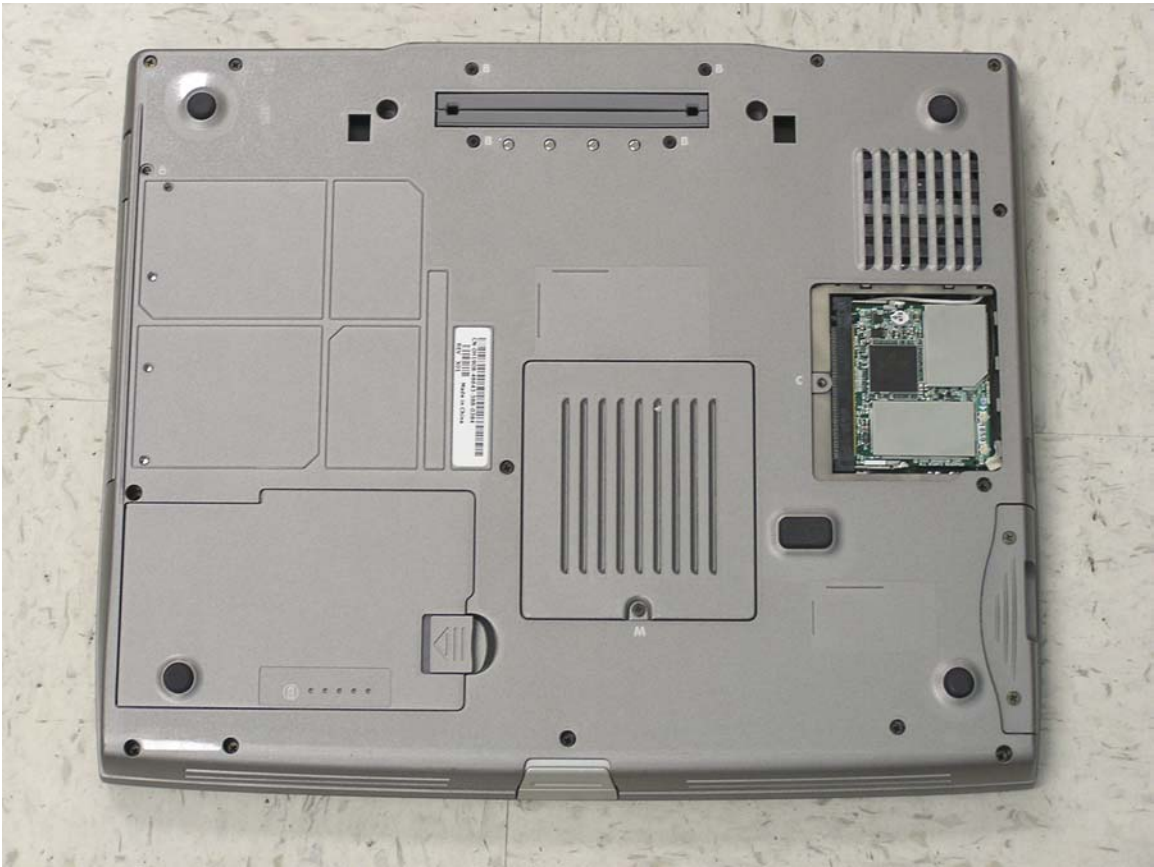
PP10L bottom view showing WLAN
