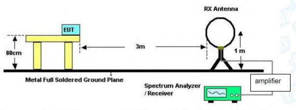
**Below 30MHz Test Setup**
