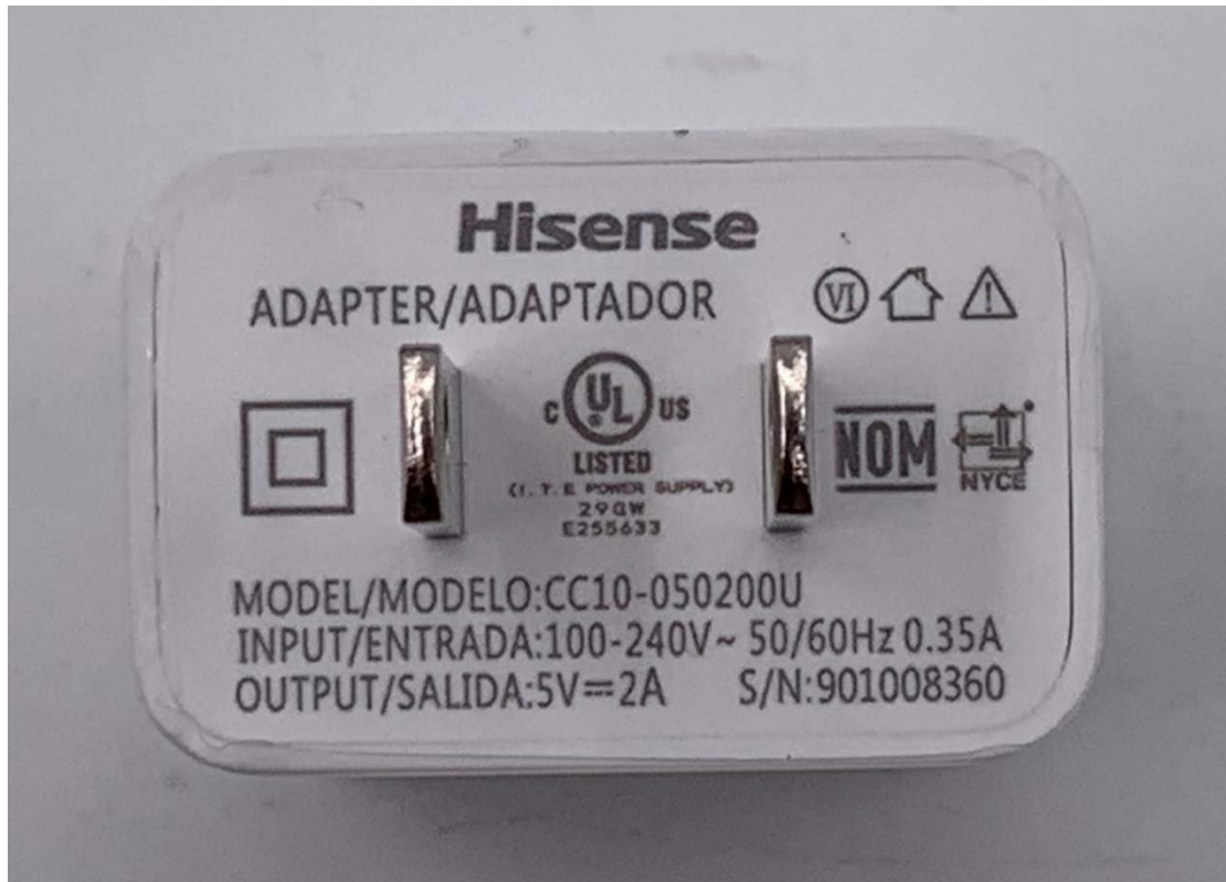
Charger View 4 (CC10-050200U made by JIANGSU CHENYANG ELECTRON CO.,LTD)
