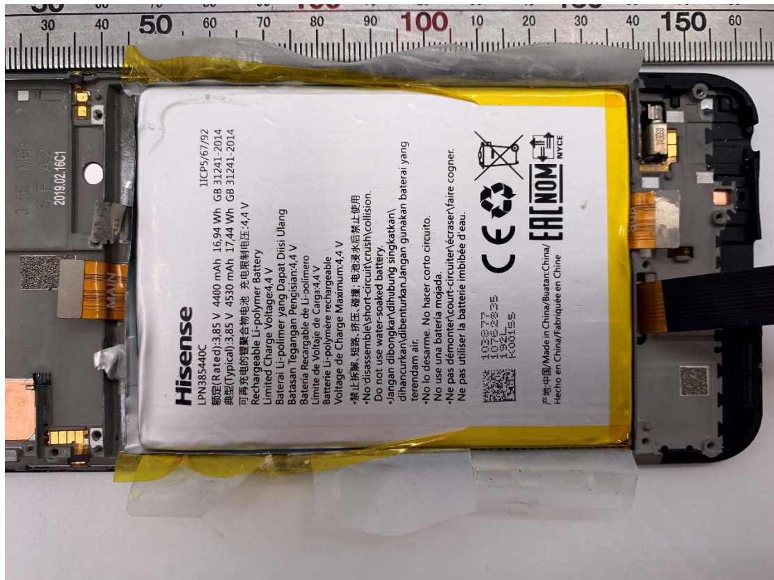
Battery View 2 (LPN385440C made by Ningbo Veken Battery Co. Ltd.)
