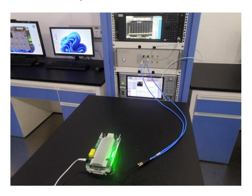
Radiated Spurious Emissions (30MHz-1GHz)
