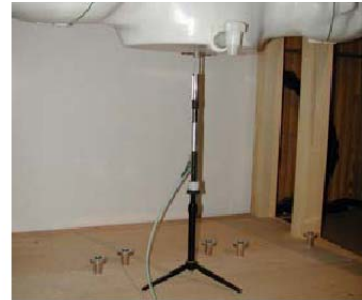
Figure 11.1 Dipole Verification Test Setup Diagram &amp; Photo
