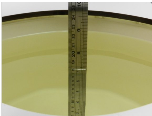
Fig 11.1 Photo of Liquid Height for Body SAR
