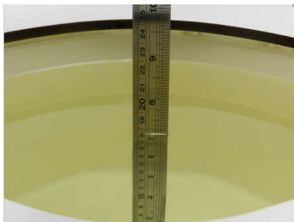
Fig 11.1 Photo of Liquid Height for Body SAR
