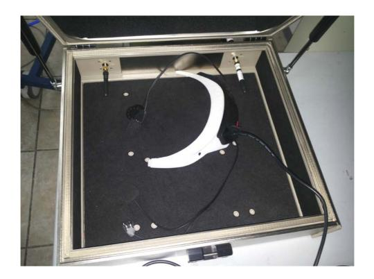
Photograph No.8 Conducted emissions on AC power lines in charging mode measurement setup
