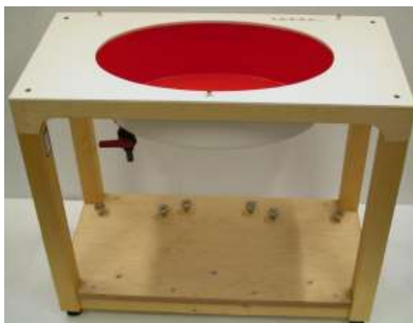
Fig.8.8 Photo of ELI4 Phantom
