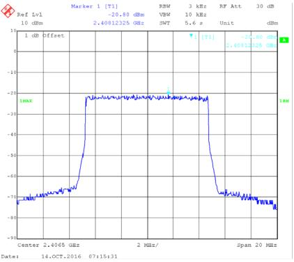
Chain 0, Power Spectral Density, Middle Channel
