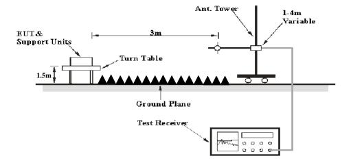
The radiated emission tests were performed in the 3 meters Semi-Anechoic Chamber, using the setup in accordance with the ANSI C63.10-2013. The specification used was the FCC 15.209 and FCC 15.247 limits.
