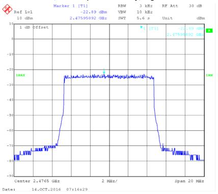
Chain 1, Power Spectral Density, Low Channel
