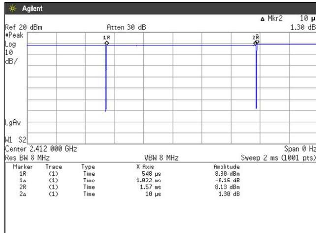
$$\text{Duty Cycle} = \text{Ton} / (\text{Ton} + \text{Toff}) = 1022[\mu\text{s}] / (1022[\mu\text{s}] + 10[\mu\text{s}]) = 99.03\%$$
