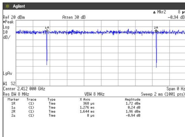
$$\text{Duty Cycle} = \text{Ton} / (\text{Ton} + \text{Toff}) = 1276[\mu\text{s}] / (1276[\mu\text{s}] + 8[\mu\text{s}]) = 99.38\%$$
