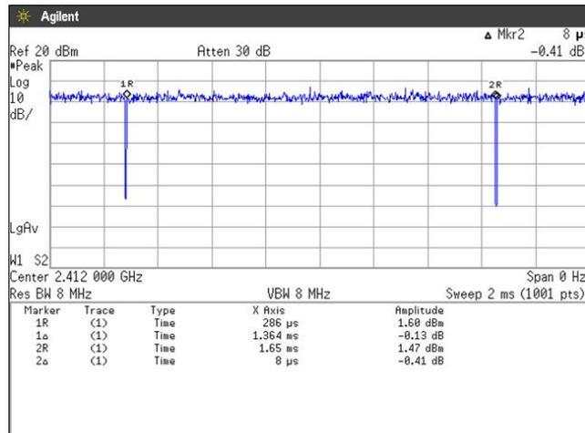
$$\text{Duty Cycle} = \text{Ton} / (\text{Ton} + \text{Toff}) = 1364[\mu\text{s}] / (1364[\mu\text{s}] + 8[\mu\text{s}]) = 99.42\%$$
