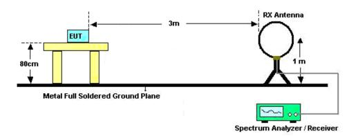
For radiated emissions from 30MHz to 1GHz
