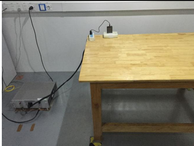
Conducted Emissions Test Setup Front View
