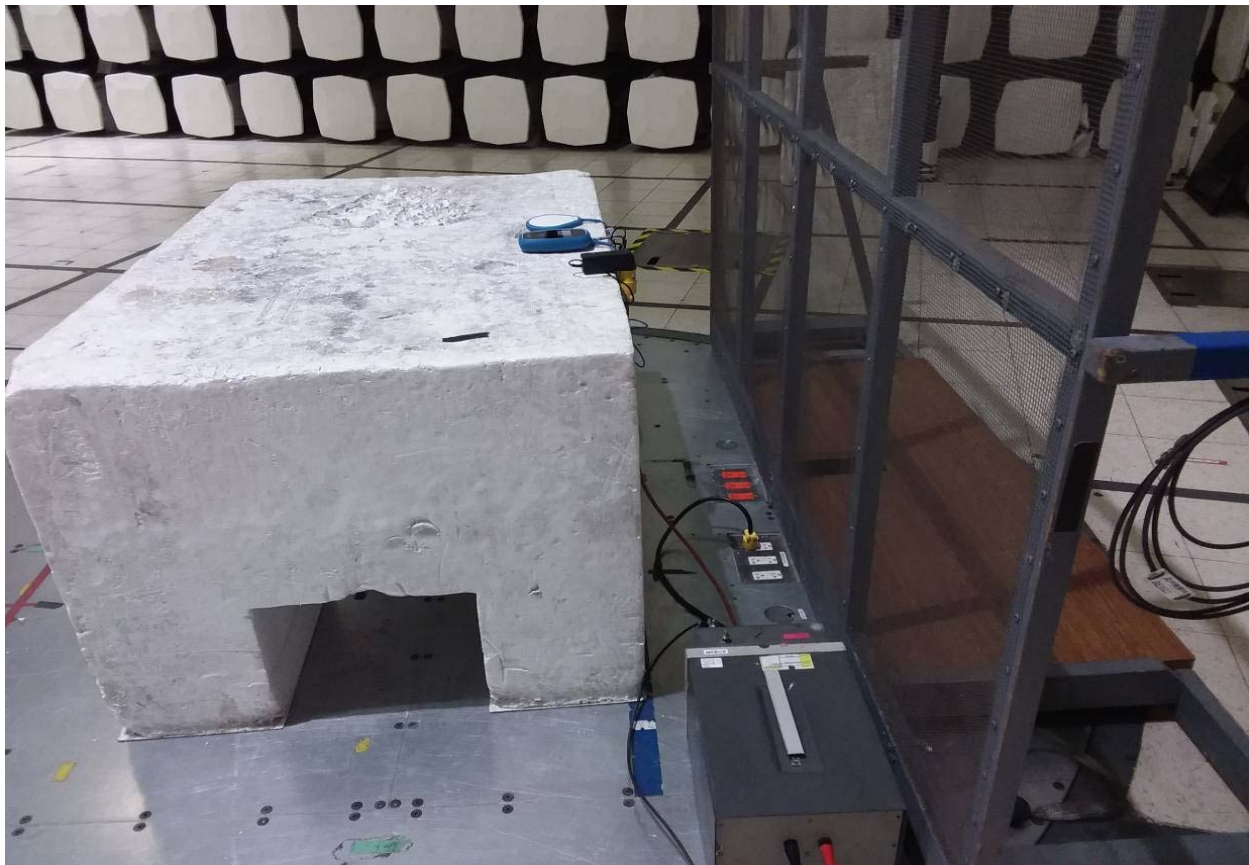
Test Configuration Photograph #1 (Conducted Emissions - Power Port)
