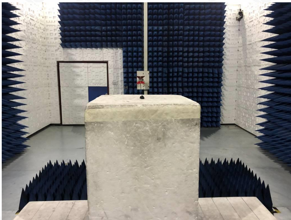
RADIATED EMISSION TEST SETUP ABOVE 1GHZ
