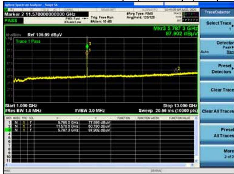
**Non-HE20, 5785MHz****P.1.P.12V Radiated Transmitter Spurs, 6 to 54 Mbps , Peak (1-10GHz)**
