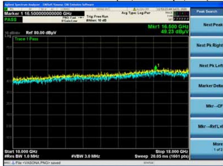
**Non-HE20, 5560MHz****P.1.P.21V Radiated Transmitter Spurs, 6 to 54 Mbps , Peak (10-18GHz)**
