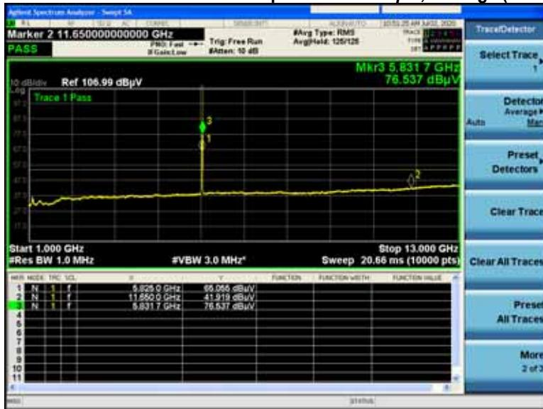
**Non-HE20, 5825MHz****A.1.A.13V Radiated Transmitter Spurs 6 to 54 Mbps , Average (1-10GHz)**
