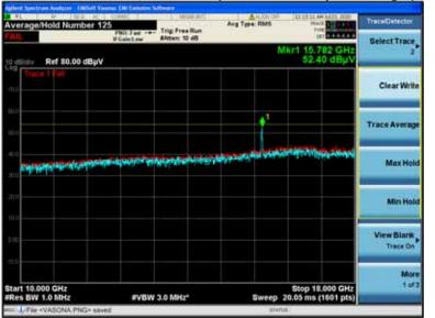
A.1.A.17V Radiated Transmitter Spurs, 6 to 54 Mbps , Average (10-18GHz)
