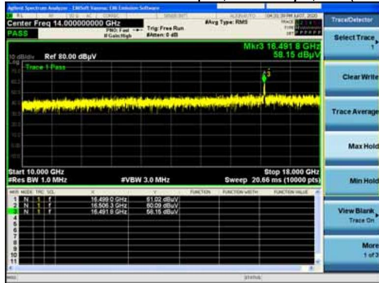
**Non-HE20, 5500MHz****P.1.P.20V Radiated Transmitter Spurs, 6 to 54 Mbps , Peak (10-18GHz)**
