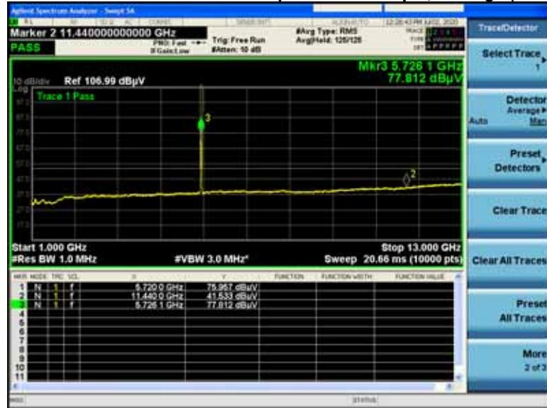
**Non-HE20, 5720MHz****A.1.A.10V Radiated Transmitter Spurs 6 to 54 Mbps , Average (1-10GHz)**
