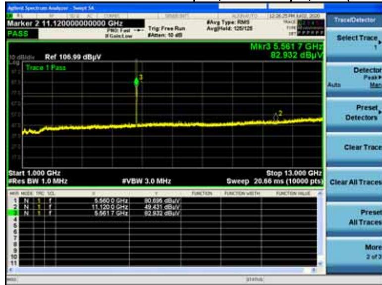
**Non-HE20, 5560MHz****P.1.P.8V Radiated Transmitter Spurs, 6 to 54 Mbps , Peak (1-10GHz)**
