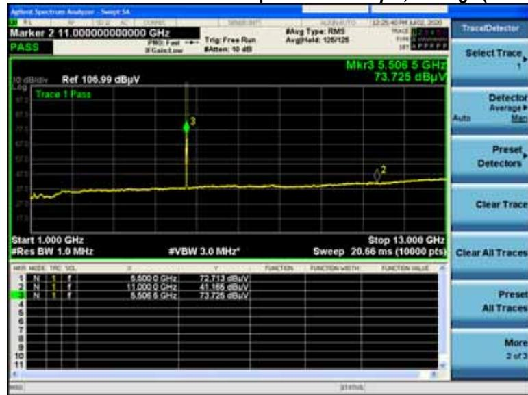
**Non-HE20, 5500MHz****A.1.A.7V Radiated Transmitter Spurs 6 to 54 Mbps , Average (1-10GHz)**
