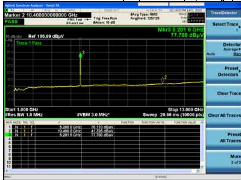
**Non-HE20, 5200MHz****A.1.A.2V Radiated Transmitter Spurs, 6 to 54 Mbps , Average (1-10GHz)**
