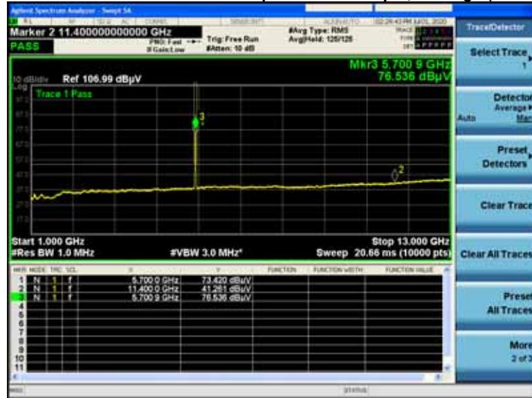
**Non-HE20, 5700MHz****A.1.A.9V Radiated Transmitter Spurs 6 to 54 Mbps , Average (1-10GHz)**
