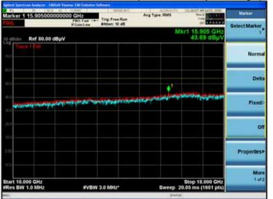
A.1.A.18V Radiated Transmitter Spurs, 6 to 54 Mbps, Average (10-18GHz)
