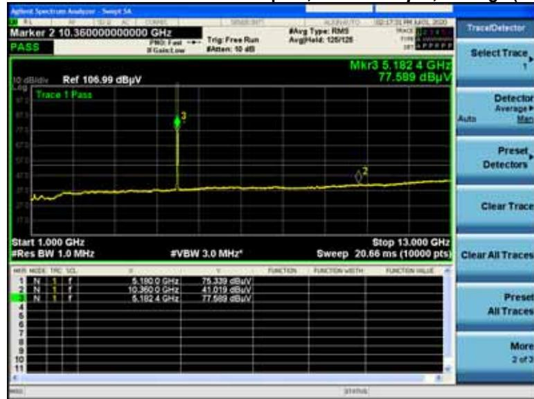
**Non-HE20, 5180MHz****A.1.A.1V Radiated Transmitter Spurs, 6 to 54 Mbps , Average (1-10GHz)**
