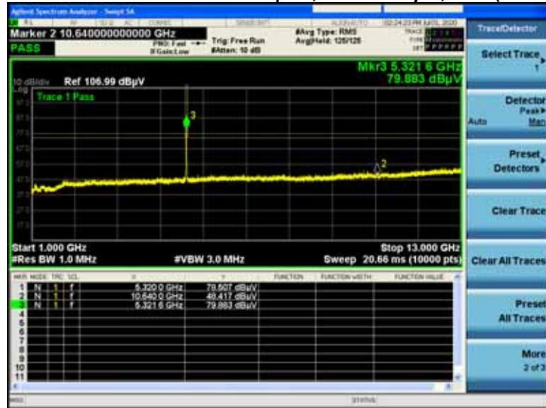
**Non-HE20, 5320MHz****P.1.P.6V Radiated Transmitter Spurs, 6 to 54 Mbps , Peak (1-10GHz)**
