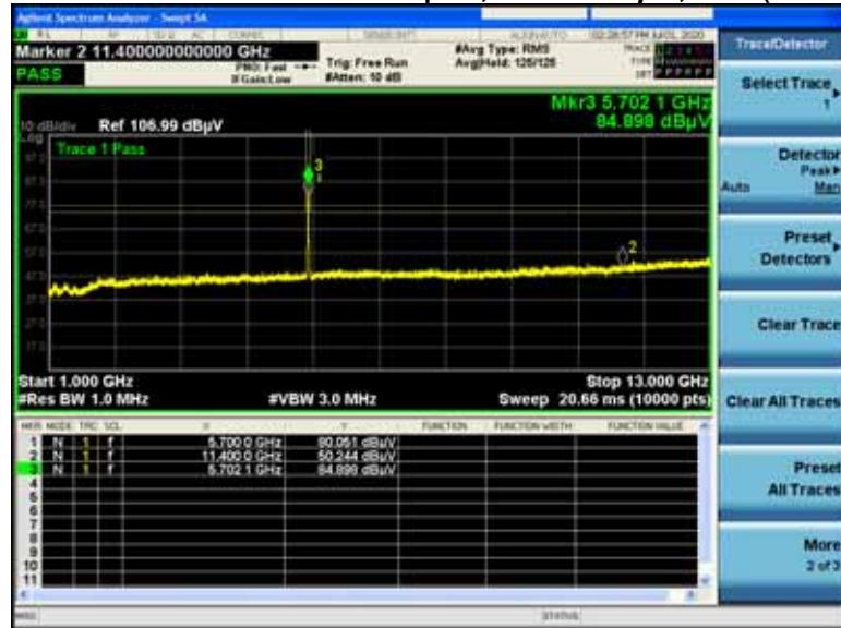
**Non-HE20, 5700MHz****P.1.P.9V Radiated Transmitter Spurs, 6 to 54 Mbps , Peak (1-10GHz)**
