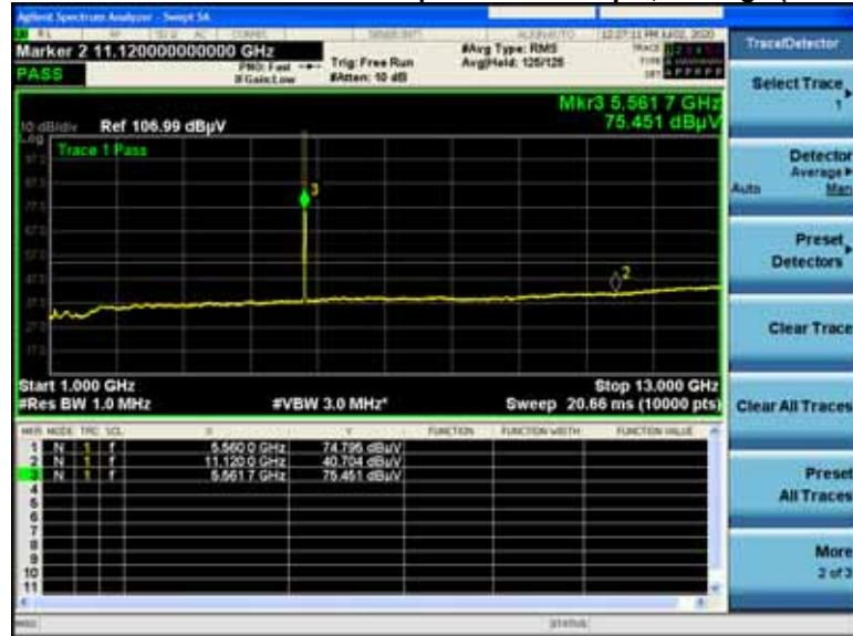
**Non-HE20, 5560MHz****A.1.A.8V Radiated Transmitter Spurs 6 to 54 Mbps , Average (1-10GHz)**
