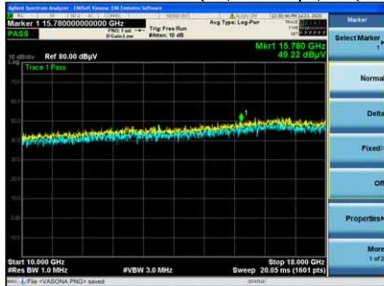
**Non-HE20, 5260MHz****P.1.P.17V Radiated Transmitter Spurs, 6 to 54 Mbps , Peak (10-18GHz)**
