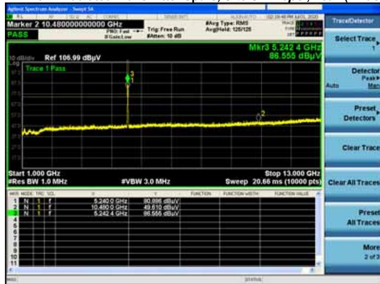
**Non-HE20, 5240MHz****P.1.P.3V Radiated Transmitter Spurs, 6 to 54 Mbps , Peak (1-10GHz)**
