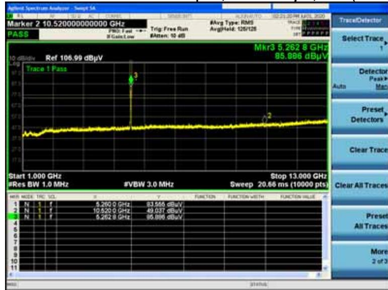
**Non-HE20, 5260MHz****P.1.P.4.V Radiated Transmitter Spurs, 6 to 54 Mbps , Peak (1-10GHz)**
