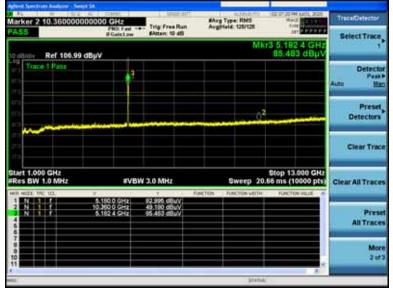
Non-HE20, 5180MHz P.1.P.1V Radiated Transmitter Spurs, 6 to 54 Mbps , Peak (1-10GHz)
