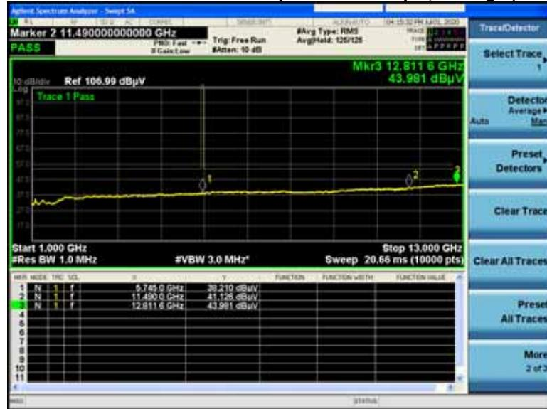
**Non-HE20, 5745MHz****A.1.A.11V Radiated Transmitter Spurs 6 to 54 Mbps , Average (1-10GHz)**
