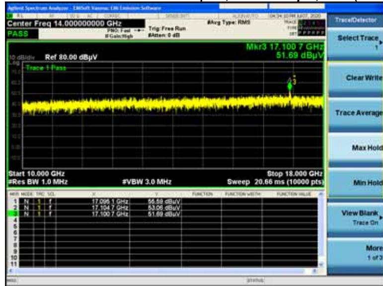
**Non-HE20, 5700MHz****P.1.P.22V Radiated Transmitter Spurs, 6 to 54 Mbps , Peak (10-18GHz)**
