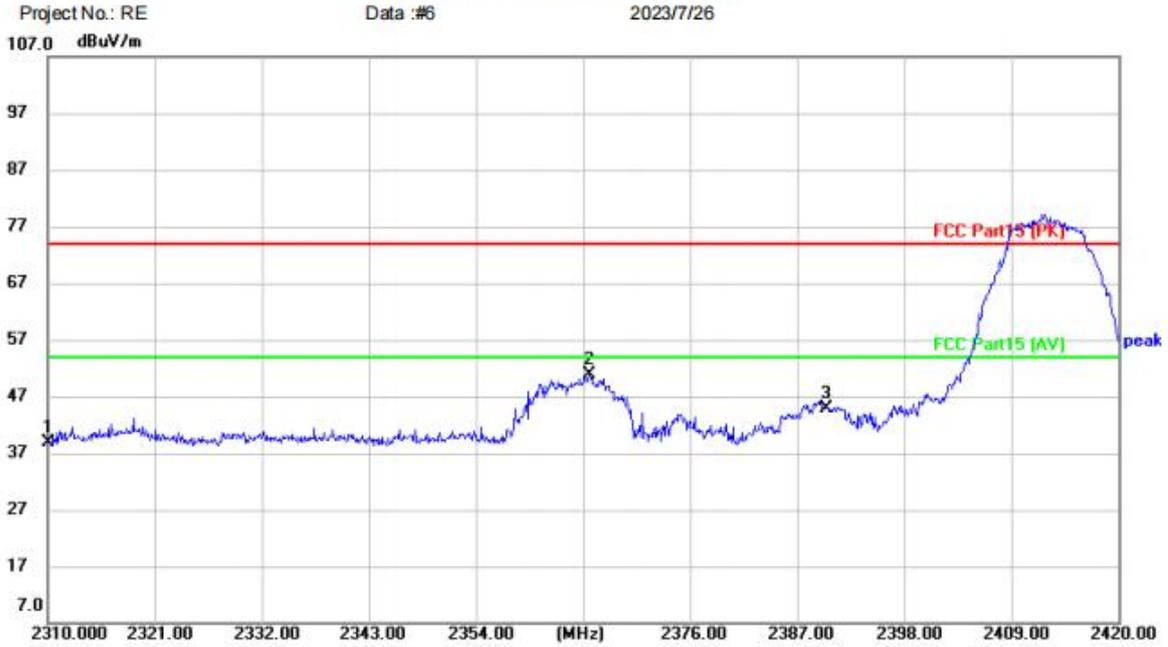
Site:      Polarization: **Vertical**      Temperature: (C)
