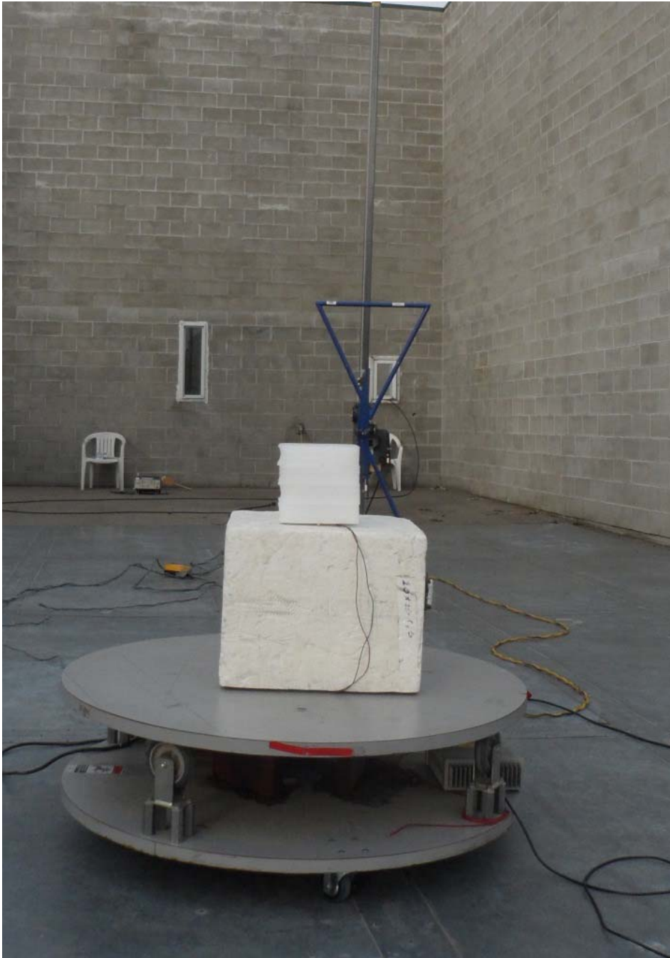
Figure E20.8 – Setup Photo – Radiated Measurements - Vertical
