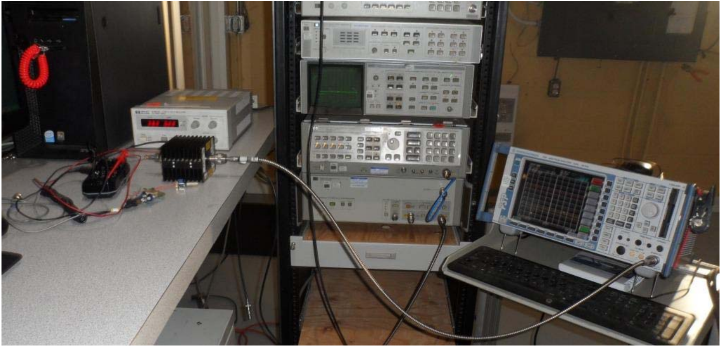
Figure E20.2 – Setup Photo – Conducted Measurements
