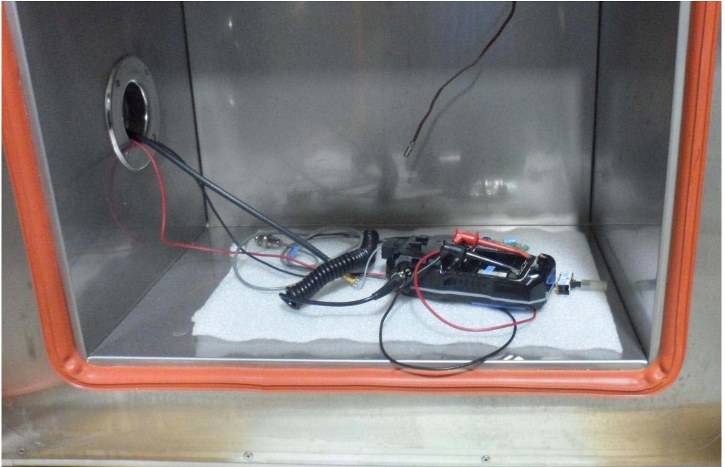
Figure E20.5 – Setup Photo – Frequency Stability Measurements
