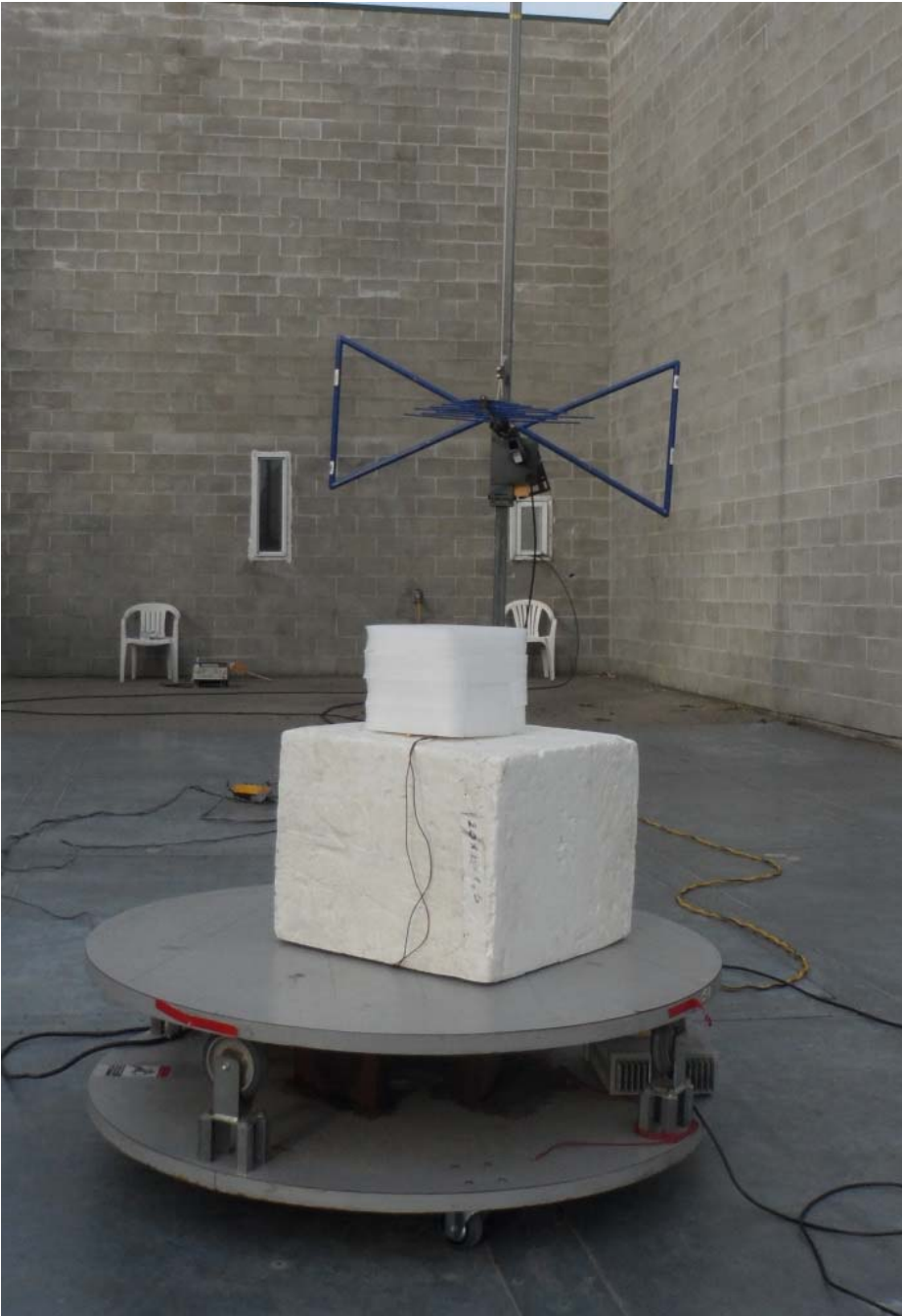
Figure E20.7 – Setup Photo – Radiated Measurements - Horizontal
