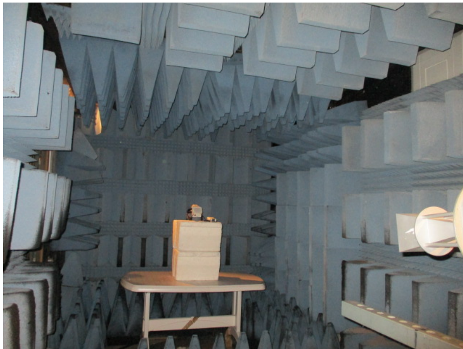
Figure 3. Radiated Emission Test, 18-26.5GHz
