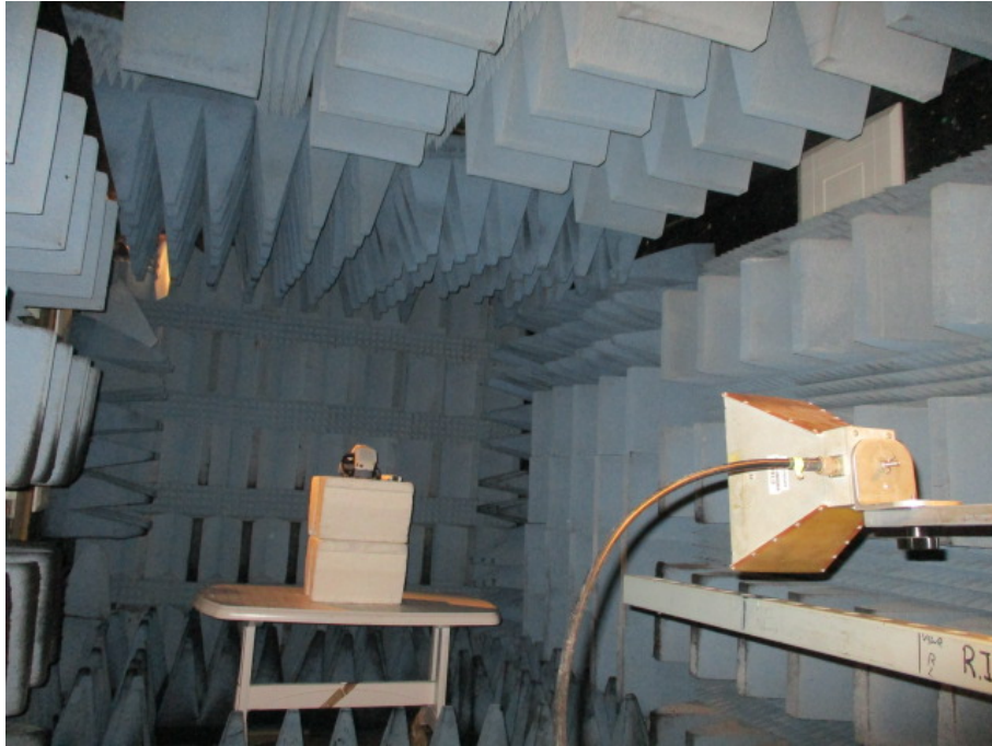
Figure 2. Radiated Emission Test, 1-18GHz
